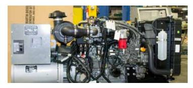
A 30kw generator is best for a Mammography or Dental Coach and a 20kw generator is typically sufficient for Health Coaches. Under-sized generators will struggle when on the road and can decrease comfort and efficiency while possibly increasing down time of your unit.
